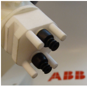
Fig. 2. The vacuum gripper used in the experiments.
